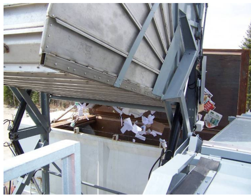
Photo 10 – Tipping of Recyclables into Compaction Trailer (Note height requirements for Transtore tipping)
